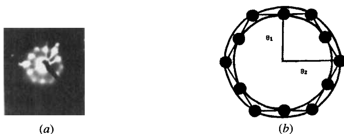
Figure 4. (a) Flat-film camera picture of the small-angle reflections of substance 1 at 155°C. (b) Scheme of the reflections.
