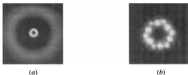
Figure 5. (a) Area detector picture of the cubic mesophase of substance 2 at 160°C. (b) Small-angle reflections of figure 5 (a).
